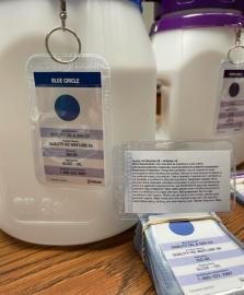
Colour-coded Labels enable accurate lubricant identification from Bulk Storage to Fill Point.
